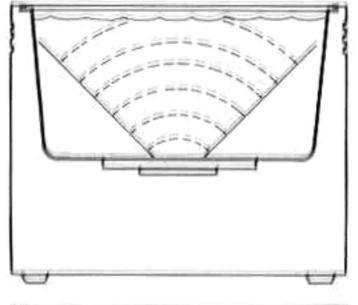
As the sound waves from the transducer radiate through the liquid in the tank, they cause alternating high and low pressures in the liquid.
