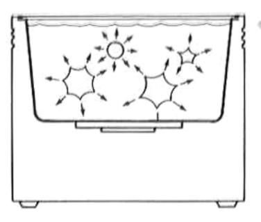
During the high pressure stage, the bubbles collapse, or "implode", releasing enormous amounts of energy. These implosions act like an army of tiny scrub brushes. They work in all directions, attack every surface and invade all recesses and openings.
