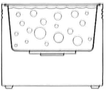
During the low pressure stage, millions of bubbles form and grow. This process is called CAVITATION, meaning "formation of cavities".
